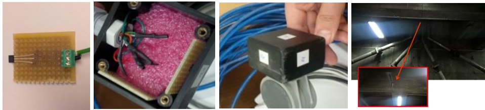
Fig. 3. Individual Hall sensor (Left), 3D Hall sensor and integrated sensor (Middle) and industrial installation (Right)
