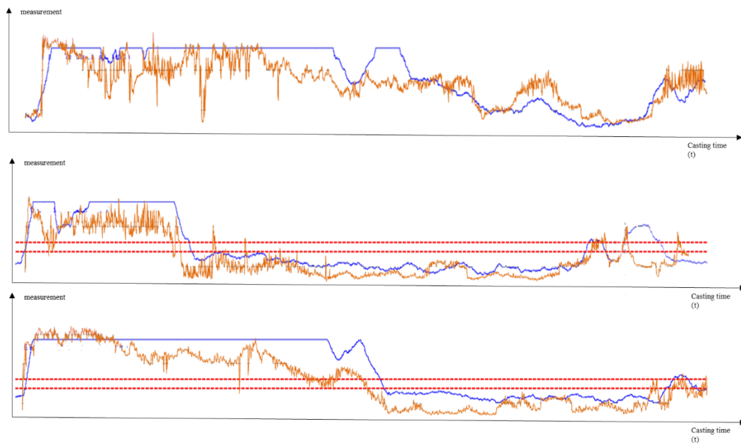
Fig. 6. Comparative analysis between Arc stability data and sound meter data in three different casts. Brown: Acoustic sensor (dB), Blue: Arc Stability index
