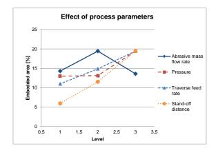
Figure 6. Effect of the process parameters on abrasive particles embedment when milling by AWJ
