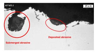
Figure 10. Submerged and deposited abrasive particles
