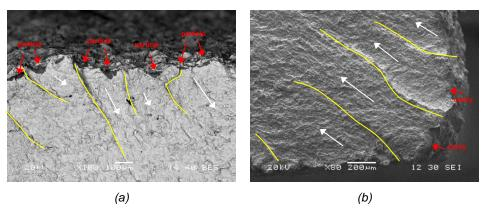
Figure 13. SEM micrograph of initiations originated at particles (Yellow line: Ratchet marks; White arrows: fatigue crack propagation direction): (a) specimen milled by AWJ; (b)specimen cleaned by PWJ
