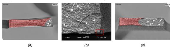
Figure 12. (a) macrograph of untreated specimen fracture surface; (b) SEM micrograph of fracture initiation of ungtreated specimen; (c) macrograph of specimen fracture surface treated by AWJ (red area: overload fracture; arrows: crack propagation direction)
