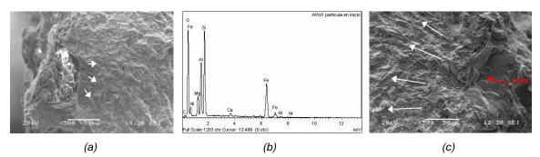
Figure 14. (a) SEM micrograph of a particle actuating a crack nucleation site in a specimen milled by AWJ; (b) EDS spectrum showing the nature of the particles at specimen treated by AWJ; (c)EDM micrograph of initiation originated at a cavity related to a particle that has been removed by PWJ.
