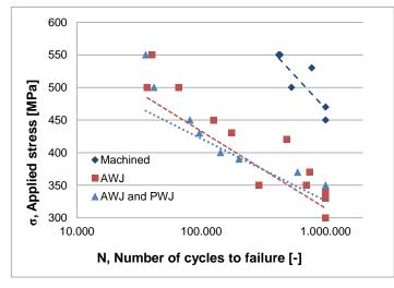
Figure 11. Maximum applied stress versus number of cycles to failure in the machined samples, and after applying the AWJ milling and the PWJ post-processing
