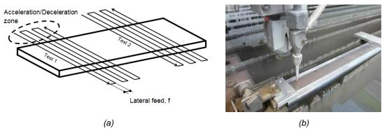
Figure 1. (a)Milling tool paths; (b) Experimental set-up;
