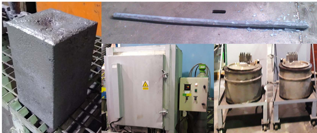
Figure 1. Type of ingots cast at lab scale, type of bars forged from the ingots (dilatometry samples and cylinders treated and investigated were cut from the forged bars), furnace and salt bath installation used in the lab scale heat treatments.
