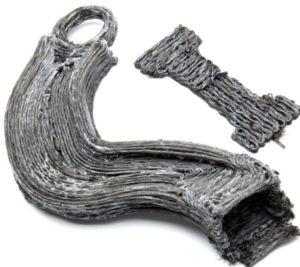
Figure 13. Continuous carbon fiber preforms manufactured using FDM technology.
