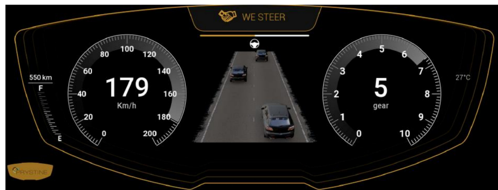
Figure 6. Example of the visual HMI, showing the level of authority and the reconstruction of the surrounding environment.
