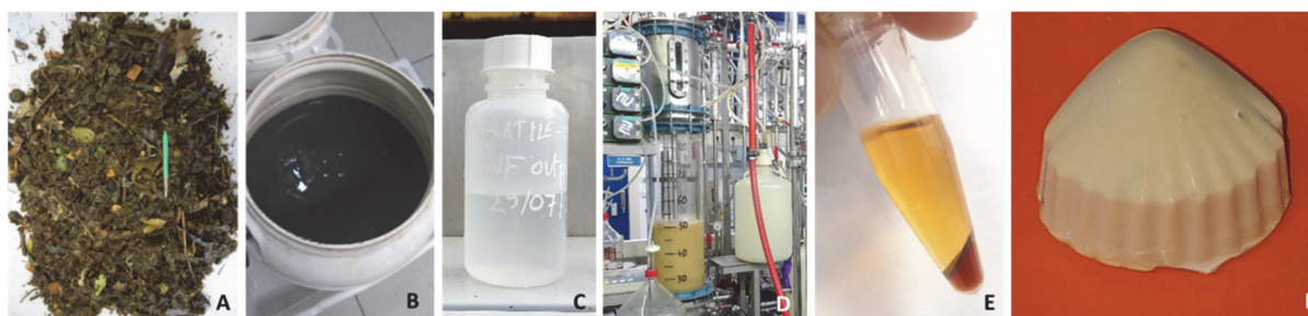
Figure 8: Transformation of VGF waste into SCO and soap A: VGF waste, B: VFA rich effluent of VFAP, C: Cleaned VFA effluent, D: Yeast fermentation using VFA rich effluents as carbon source, E: SCO extraction from yeast biomass, F: biowaste derived soap
