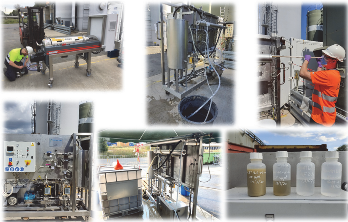
Figure 9: Validation of centrifugation, ultra- and nanofiltration and reverse osmosis at pilot scale
