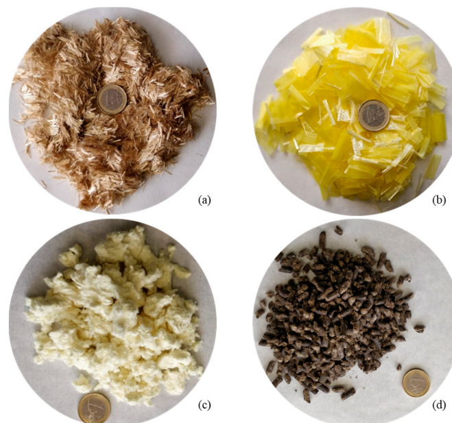
Figure 2. Fibers used in the study: (a) Aramid fiber (ARA); (b) Aramid-Polyolefin fiber (ARA-POL); (c) Aramid Pulp (PULP); (d) Cellulose fiber (CELLU).
