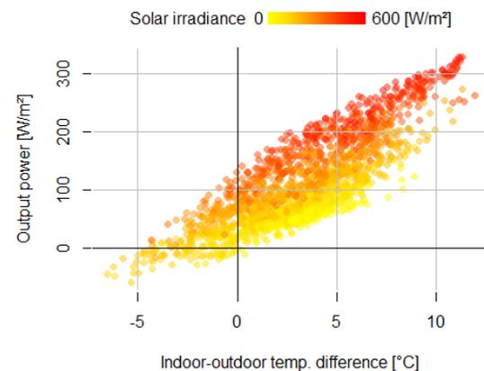
**Fig. 5.** Output power in the cavity vs Indoor-outdoor temperature difference. Hourly-averaged values.
