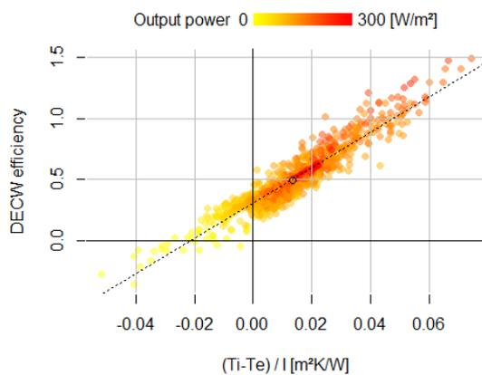
**Fig. 7.** Efficiency of the solar collector as defined in eq (3). Hourly-averaged values
