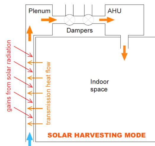
**Fig. 1.** Schematics of system operation in solar harvesting mode.
