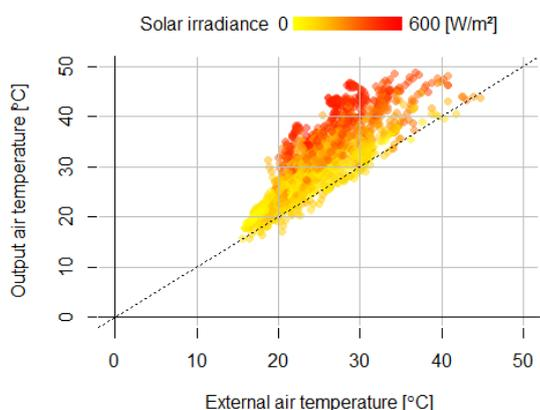
**Fig. 4.** Inlet-outlet temperature gain in the cavity.
