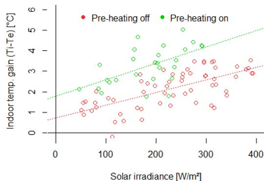
**Fig. 3.** Daily averaged indoor-outdoor temperature gain, with and without pre-heating of ventilation air.
