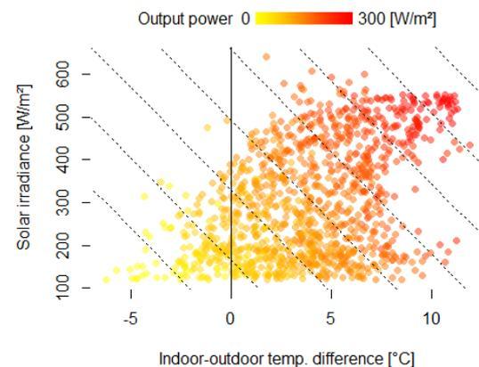
**Fig. 6.** Output power as a function of solar irradiance and temperature difference. Hourly-averaged values.
