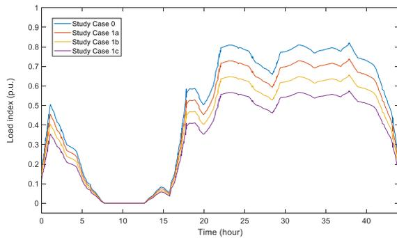
**Figure 4.** WTSU transformer load index for Study Case 1.
