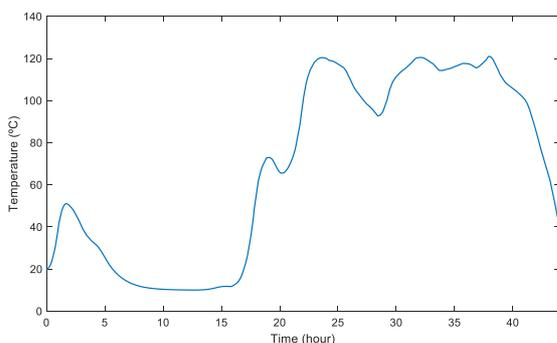
**Figure 2.** Hot-spot temperature for base case.
