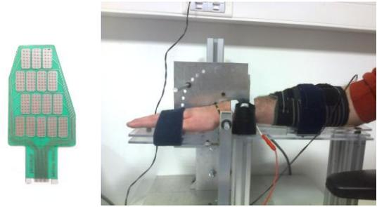
Figure 1. Multi-field electrode and experiment set-up.
