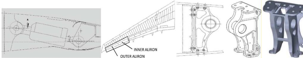
Figure 2. (left) common design and assembly (right) new bionic part.
