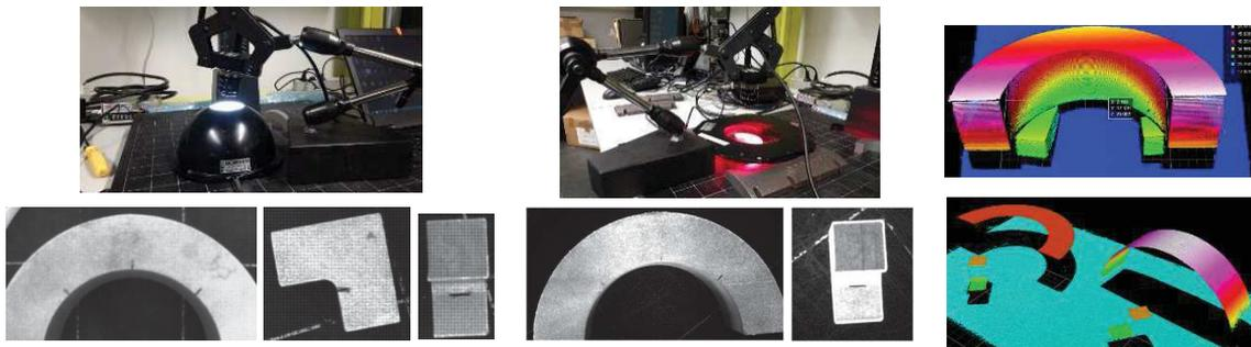
Figure 8. Images obtained with: (Left) Domo (centre) Darkfield (left) Laser Triangulation based 3D vision system
