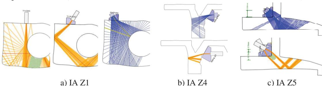
Figure 10. Results from simulations identifying non-inspectable areas (in green).
