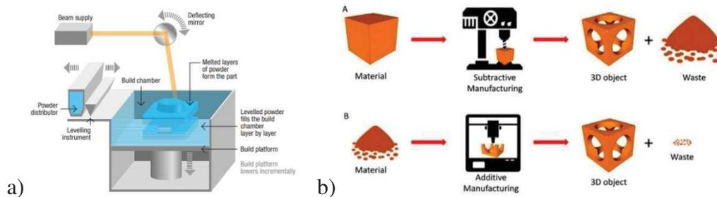
**Figure 1. a) LBM process (2); b) Differences between CNC and ALM (4)**
