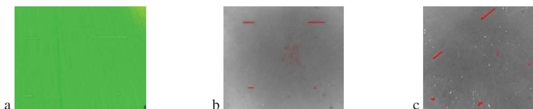
**Figure 3. a) Structured Light, b) Domo (+ Halcon), c) Darkfield (white illumination + filter) Laser Triangulation images are not added due to negative results obtained**
