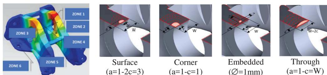
**Figure 6. Critical zones and shape and dimensions (mm) of each type of defect**
