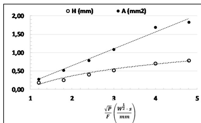
Fig. 2. Area (linear) and height (logarithmic) trend, 4-stream nozzle, R50%, P=2500W, Focusing screw 10. Y-axis: area and height values.
