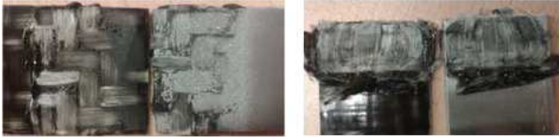
Fig. 7. Failure mode (a) PA6+47%GF-DC01; (b) PA6+47%GF-ALMg3.
