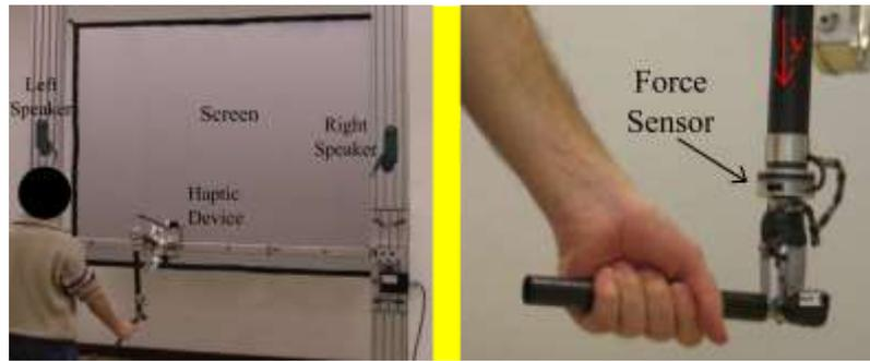
Fig. 2. On the left, the experimental setup comprising of a projector screen, the six-DOF LHIFAM haptic device and a pair of speakers. On the right, users hold the LHIFAM's stylus in the form of force grip.
