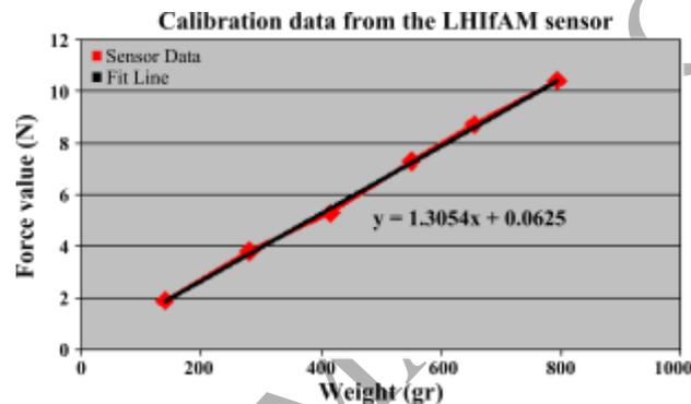
Fig. 3. Line of best fit to describe the LHIFAM's force sensor response.
