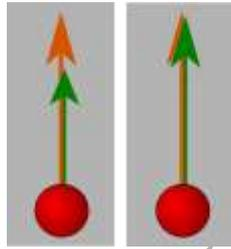
Fig. 4. Punctual information using visual feedback; on the left, the user (green arrow) is applying less force than the target (orange arrow); on the right, the user (green arrow) is applying the same level of force as the target (orange arrow).
