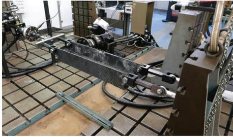
Fig. 5. Durability test set-up of Subframe demonstrator
