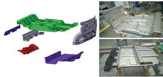
Fig. 7. Evolution underbody demonstrator
