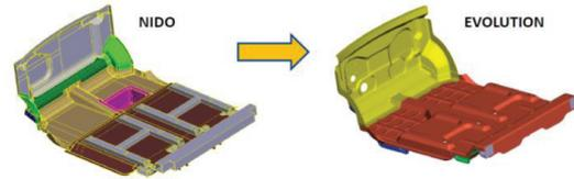
Fig. 6. Nido underbody concept (left) and Evolution underbody demonstrator (right)
