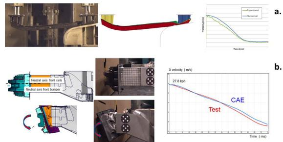
Fig. 3. AZT test/CAE (a) and calibration test/CAE (b)
