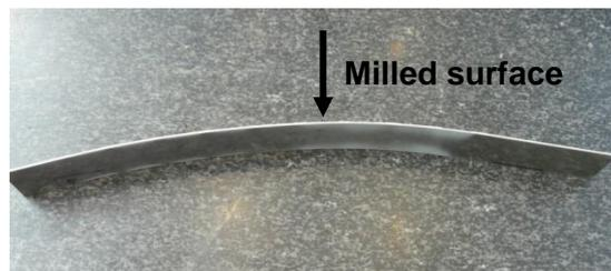
Figure 5. Curvature of the samples milled by AWJ
