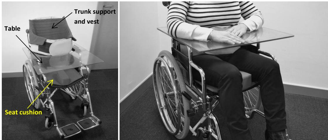
Figure 3: Final prototype of the Wheelchair Posture Support Device. Left: WPSD installed in a wheelchair – trunk support containing Varstiff® covered with a 'vest', seat cushion with 'pommel', transparent arm support table. Right: Person seated with a correct posture due to WPSD and transparent table.
