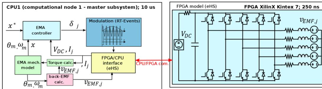
Figure 3 General diagram of the implemented Real-time multiphase EMA landing gear platform in OP4510.
