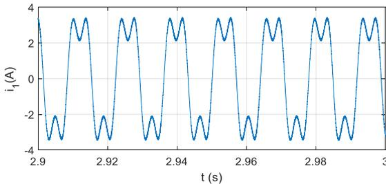
Figure 7: Phase U current during maximum load conditions.
