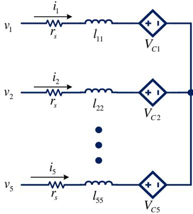
Figure 1: Motor model in the natural reference frame [5].
