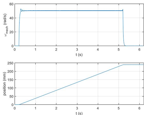
Figure 4: Speed and position control during the EMA landing gear extension.
