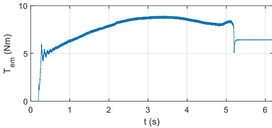
Figure 5: Electromagnetic torque produced by the fundamental and third harmonic components.
