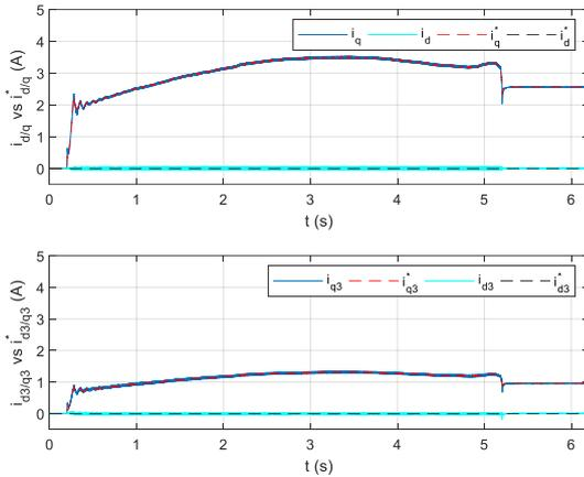
Figure 6: Fundamental and third harmonic d- and q-axis current control.
