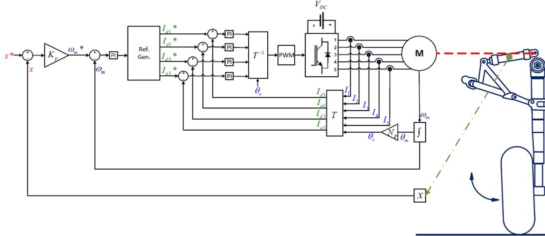
Figure 2 General diagram of the position control of the landing gear EMA during normal operation.
