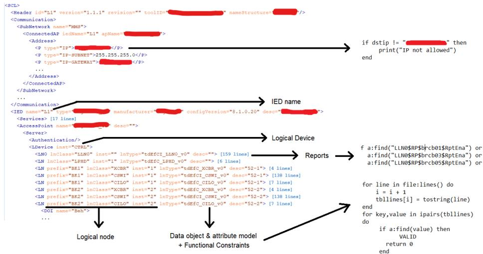
Figure 4: Mapping between SCL files and Lua detection rules
