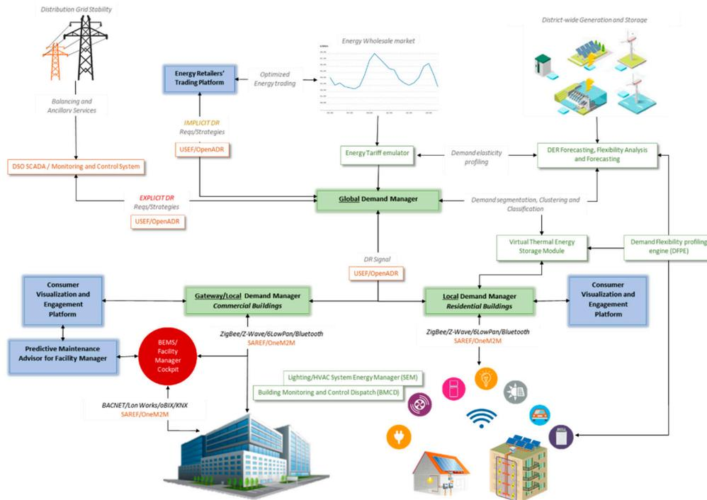
**Figure 1.** Detailed representation of the architecture of the solution.
