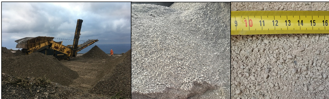
Fig. 12. Limestone concrete fines (RCLG) from the Gutram valorisation plant used in the pilot test.
