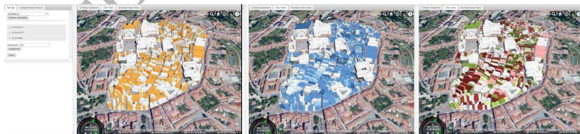
Figure 7: Visualization of the results for the ECM6 (Diffusion closed interior insulation). From left to right: Negative HIA, positive HIA and balanced HIA index
